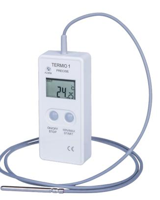
**Temperature loggers TERMIO-1/2** are intended for temperature measurements in ranges -100°C to + 300°C depending on external probe. **Termio 15** is intended for temperatures in ranges -30 to + 70 °C. The devices have memory that allows them to save 32 thousand measurements. The logger may be used to monitor the temperature during the storage and transport of vaccines, medicine, and food, as well as production and warehousing, etc.
