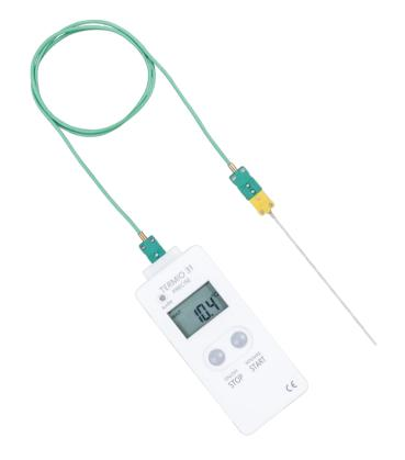
Temperature logger TERMIO-31 is intended for temperature measurements in ranges -200°C to + 1400°C depending on external probe. It is equipped with a thermocouple mini socket and memory that allows it to save 32 thousand measurements. The logger may be used to monitor the temperature during the storage and transport of vaccines, medicine, and food, as well as production and warehousing. etc.
